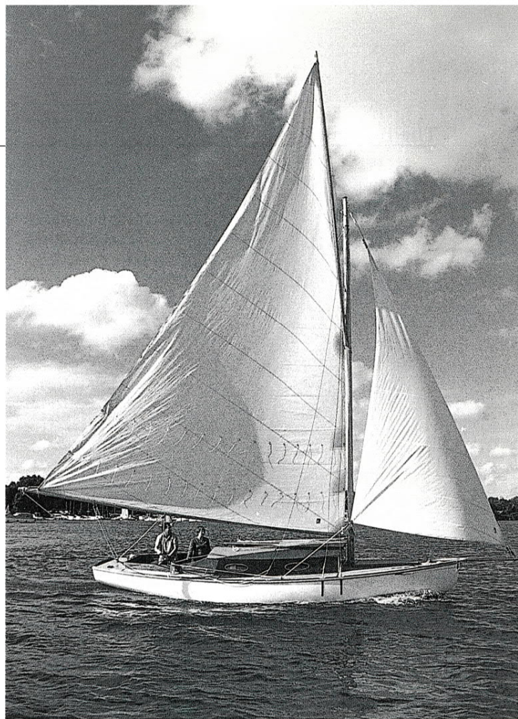
The Strider prototype for a modern 25' (7.6m) Broads yacht designed for Kingsley Farrington. Photograph: Andrew Wolstenholme.
