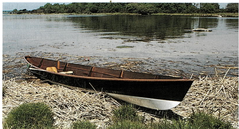
The prototype of the Sprite, a double chine plywood rowing skiff, now produced as a kit by Chippendale Craft.
