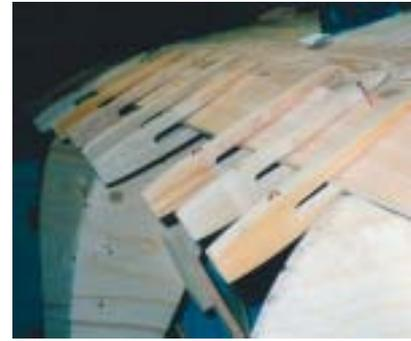
To ensure a nice tight fit at the lands – the plank overlaps – I made lots of peg clamps. I waterproofed the seams between the garboards and the keel and at the hood ends with Sikaflex, the rest were dry-fitted and on launching, there wasn't one leak!
