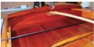
**Above:** Instead of a sheethorse, I fitted a 'bridge' between the quarter knees to support a rail. The bridge is profiled to clear the tiller and there is a sculling notch which doubles as a mast support for trailing.
