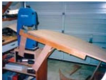
*In order to saw the right bevels on edges of the transom, I made up this jig for the bandsaw to hold the mahogany at the correct angle.*
