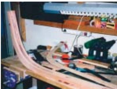
*The apron, laminated from 3 layers of mahogany in 3 sections with an inner full-length veneer to hide the joints, was glued with resorcinol.*
