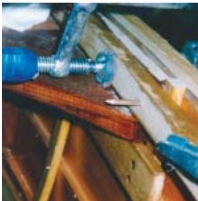
**Above:** When the varnish was dry, the timbers were re-fitted: rivetted through the lands and screwed down to the hog, taking great care that they were all at 90° to the hog. Note the wedges which support the timbers either side of the hog.
