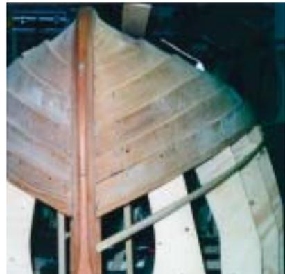
How did I do it? After roving up, I temporarily fixed a round batten on the marks for the next plank which acted as a guide for the plane when planing the bevel. A supporting bar, fixed to the plane, slid along the round batten.
