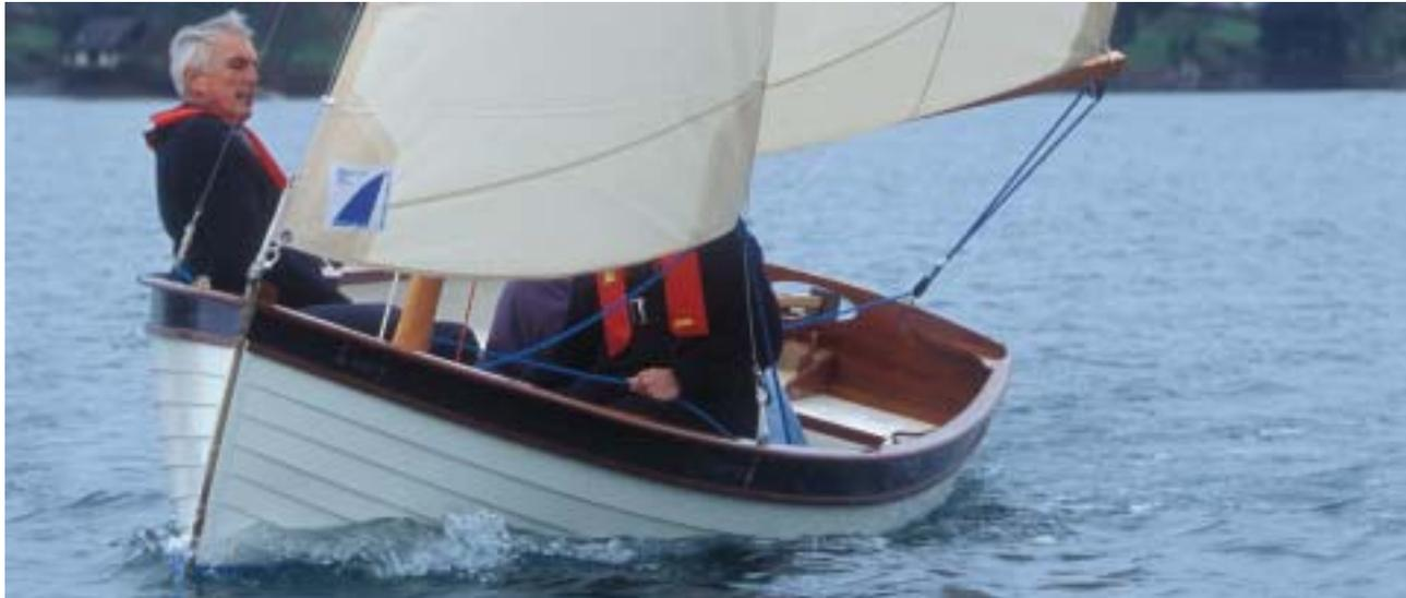
where there is ample space for the crew's feet on the slatted larch bottom boards. The wooden centreboard and the blade of the lifting rudder are aerofoil in cross section, ensuring maximum efficiency, with the up- and downhaul lanyards on the rudder leading through the attractive elliptical hole in the transom which houses the tiller.
